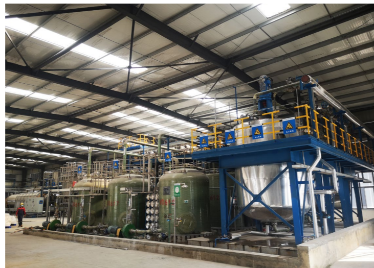
Picture: 1,000-ton iron phosphate process pilot plant
